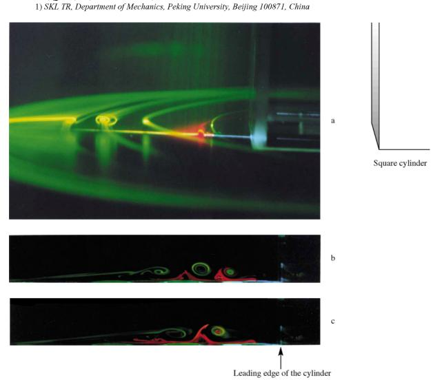
2.a shows the pattern of a juncture flow in the front of a square cylinder mounted on a flat plate. The horseshoe vortices shed from the separated shear layer consecutively, and lastly merge each other then form a main horse-shoe vortex that is closest to the cylinder.
